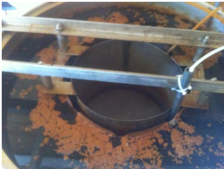
Figure 3. Top interior of redesigned Site A pilot bead filter
