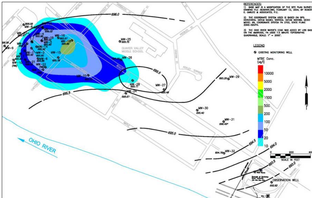
Figure 14. MTBE Plume and Apparent Capture Zone of Groundwater Cut-off Remedy.
