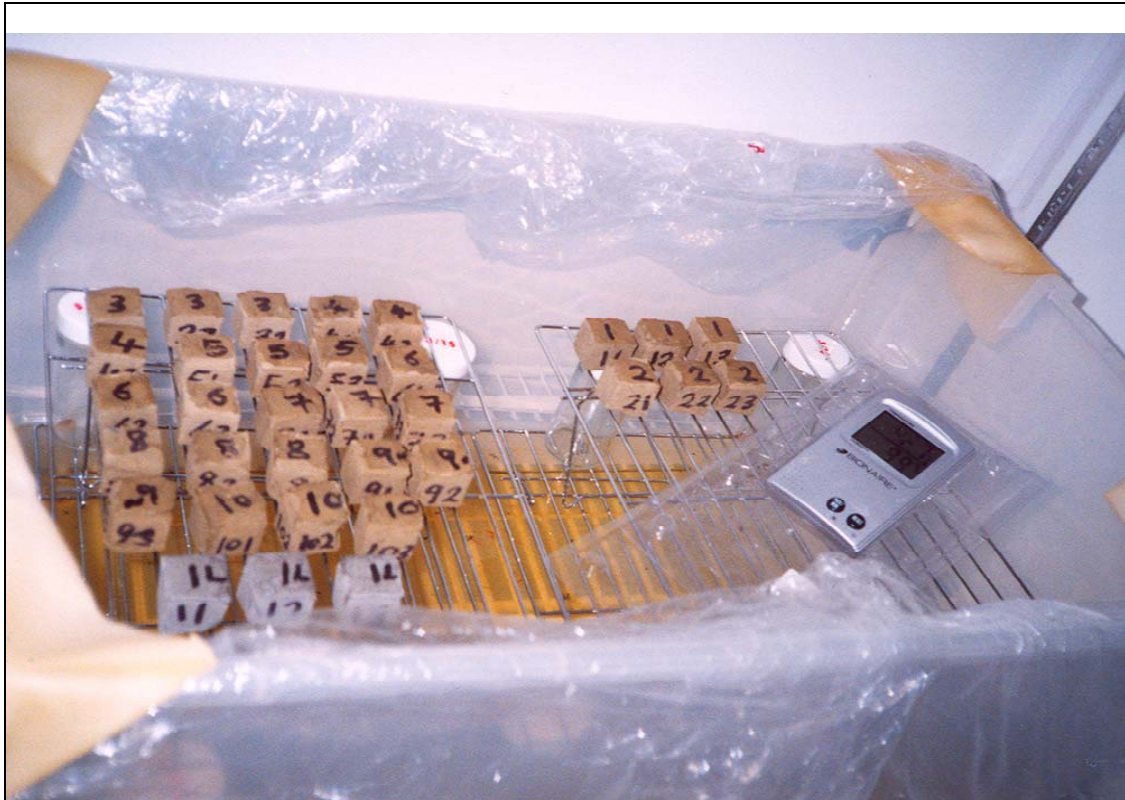
Figure 1. Tailings specimens inside the moisture chamber
