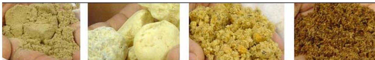
Figure 1. Appearance and relative size of the different bulking agents used in this study. From left to right: fill sand, gravel, sharp sand and sawdust. The length of each picture corresponds to a length of 7.7 cm.
