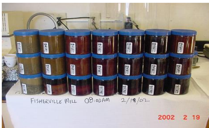
Figure 21. Sodium Permanganate Bench-Scale Treatability Testing
