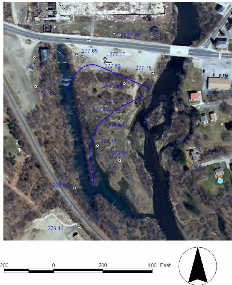
Figure 5. Potentiometric contours (277.6 and 277.4 feet) based on water elevations measured in deep overburden monitoring wells on July 16, 2001.
