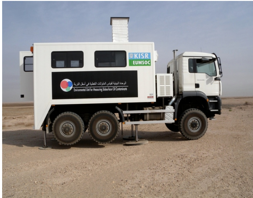
Figure 1. The mobile LIF/CPT lab developed at KISR and identified as the Environmental Unit for Measuring Subsurface Oil Contaminants (EUMSOC). In this view the vehicle is raised on the self-lifting jacks, and the lowered LIF probe is seen in between the vehicle's front-rear wheel and the front lifting jack.
