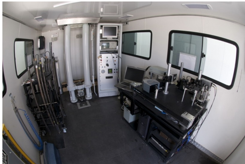
Figure 2. View inside of EUMSOC showing the laboratory's main components. From the right: the optical bench incorporating the laser source, detectors and optics. The CPT control, output displays and the main press mechanism are at the center. On the left is the carriage-holder of the probe segments.
