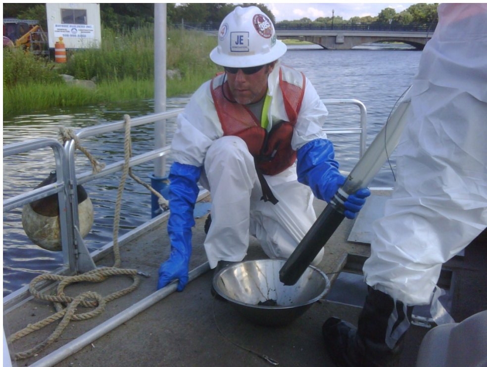
Figure 4. Collecting a Sediment Core from New Bedford Harbor.
